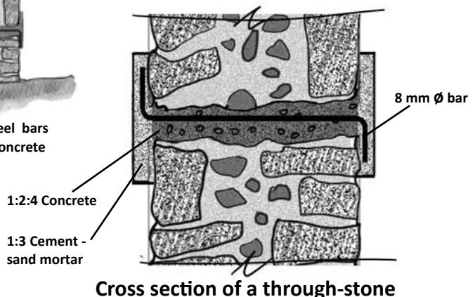
mimic good construction practice for stone masonry where long stones (bonding stones) are provided. The effectiveness of through-stones in new construction is discussed in Chapter 3.
