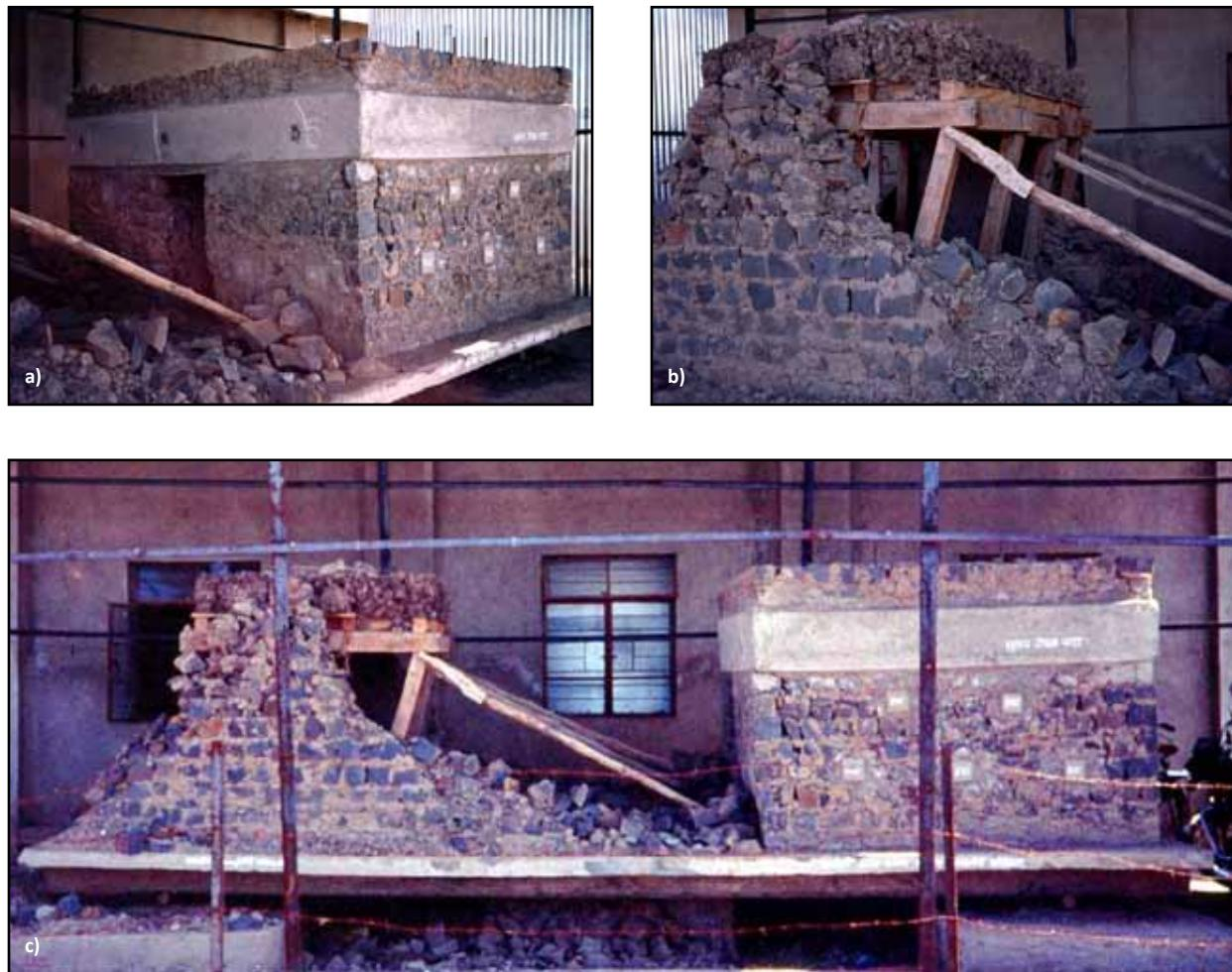
**Figure 4.1** Verification of seismic retrofitting methodology for stone masonry buildings through shake-table testing: a) strengthened (retrofitted) model, b) unstrengthened model after testing, and c) models at the end of the experiment (unstrengthened model shown on the left) (source: GOM 1998)
