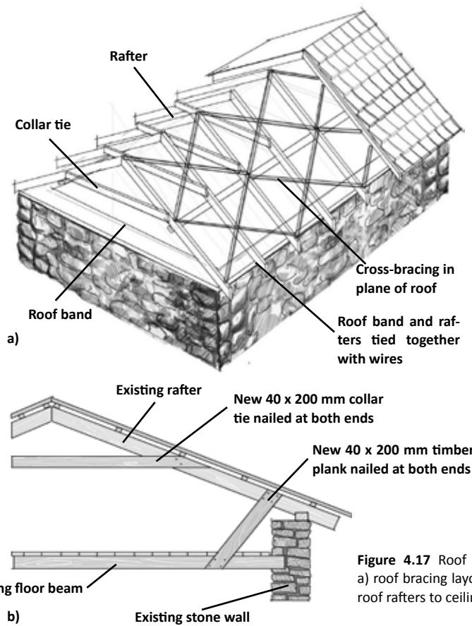
Figure 4.17 Roof bracing details:
