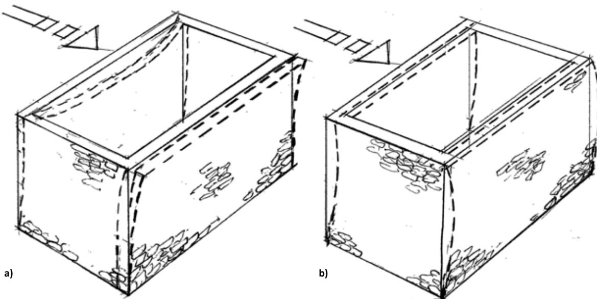
**Figure 2.5** Masonry building during earthquake shaking: a) loosely connected walls without slab at the roof level, and b) a building with well-connected walls and a roof slab (source: Tomazevic 1999)
