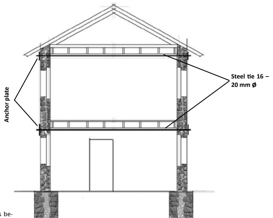
Figure 4.3 A vertical building elevation showing ties beneath the floor level (adapted from: Tomazevic 1999)
