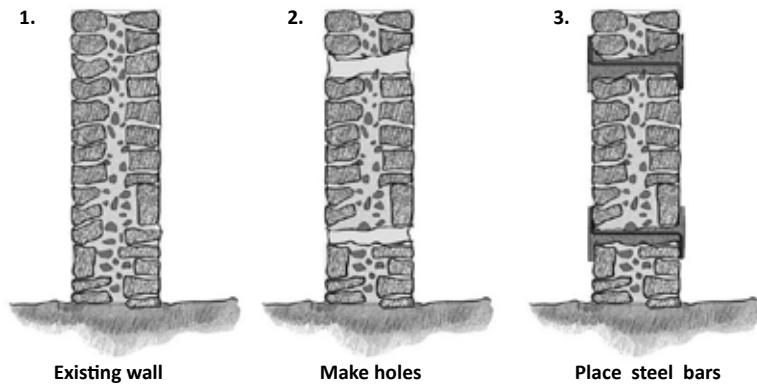
**Figure 4.18** Procedure for the installation of through-stones (source: GOM 1998)
