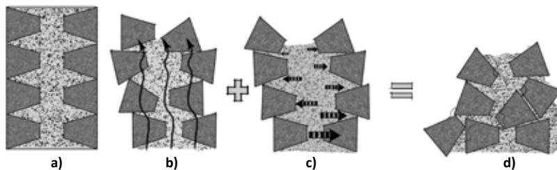
**Figure 2.21** Delamination of stone masonry walls: a) two-wythe stone wall with a rubble core; b) stones are displaced due to vibrations; c) internal lateral pressure due to rubble fill increases, and d) the wall collapses (source: Meyer et al. 2007)
