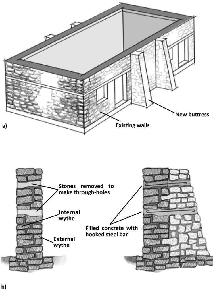
**Figure 4.28** Strengthening an existing stone wall with buttresses
