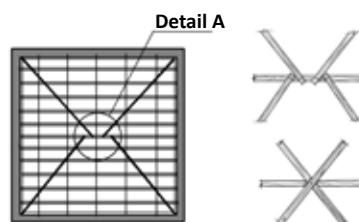
Figure 3.36 Details of floor and roof bracing
