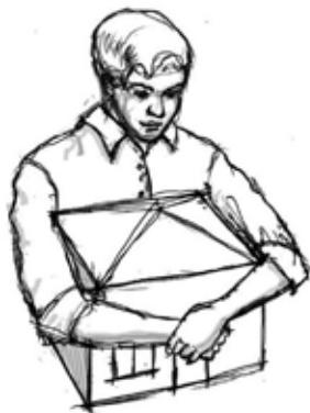
**Figure 3.7** A seismic band acts like a belt (adapted from: GOM 1994)
