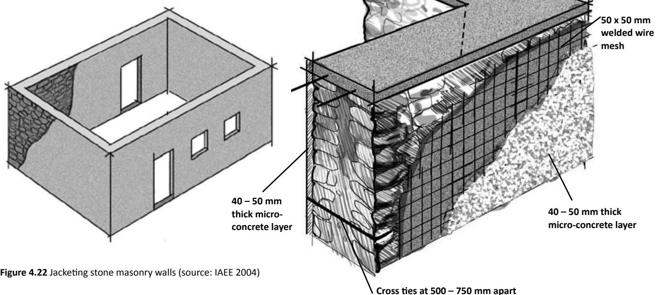
Figure 4.22 Jacketing stone masonry walls (source: IAEE 2004)
