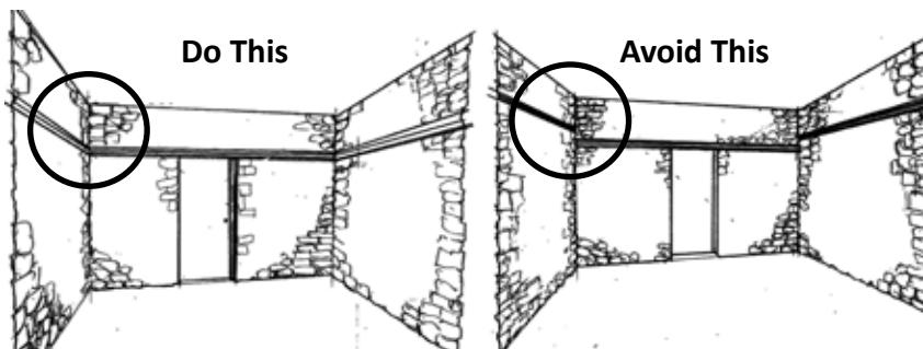
**Figure 3.10** Seismic bands should always be continuous; an offset in elevation is not acceptable (adapted from: GOM 1998)
