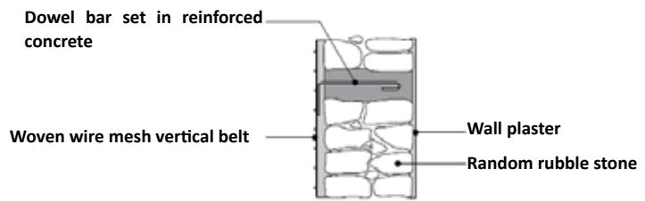
**Figure 4.25** Single-sided jacketing showing steel dowels
