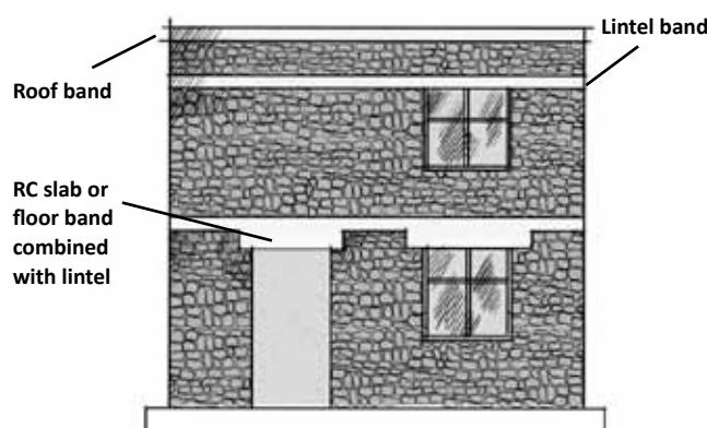
**Figure 3.12** Merging RC floor and lintel bands
