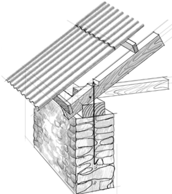
Figure 3.35 Tying roof rafters at the eaves level
