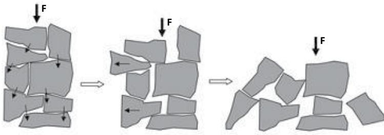
**Figure 2.36** Detail of wall failure caused by irregular stones (source: Bothara and Hiçyilmaz 2008)
