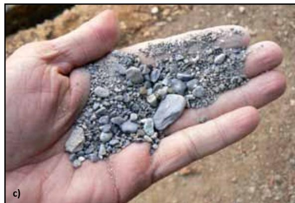
Figure 3.42 Sand for different uses: a) fine sand for plaster construction; b) coarse sand for mortar and concrete construction, and c) excessively coarse sand (photos: Smart Shelter Foundation)
