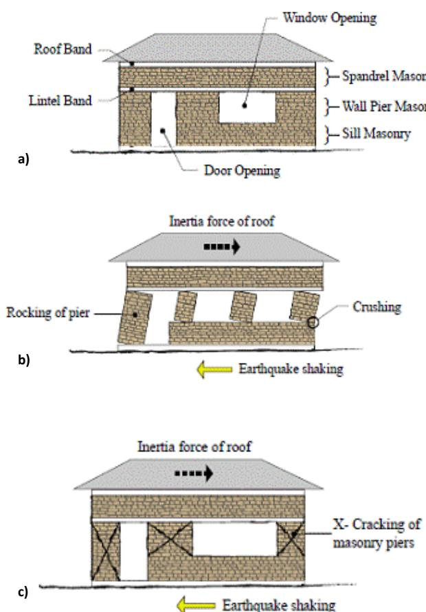
**Figure 2.33** In-plane damage of stone masonry walls: a) typical wall with openings; b) rocking failure, and c) diagonal shear cracking (adapted from: Murty 2005)
