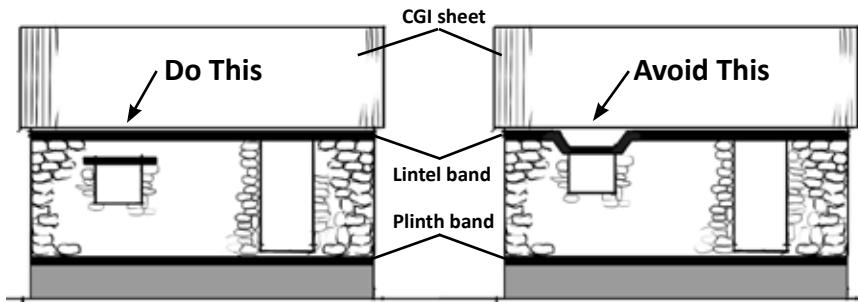
**Figure 3.11** RC seismic bands should always remain level without any dips or changes in height (adapted from: GOM 1998)
