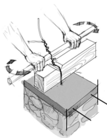
Use double 3 mm wire to anchor the joist and make a notch to prevent movement in the beam.
