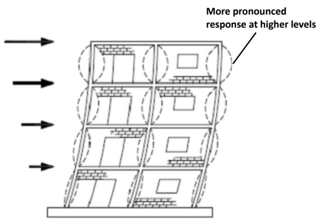
**Figure 2.24** Out-of-plane vibrations of stone masonry walls are most pronounced at the top floor level (source: Tomazevic 1999)
