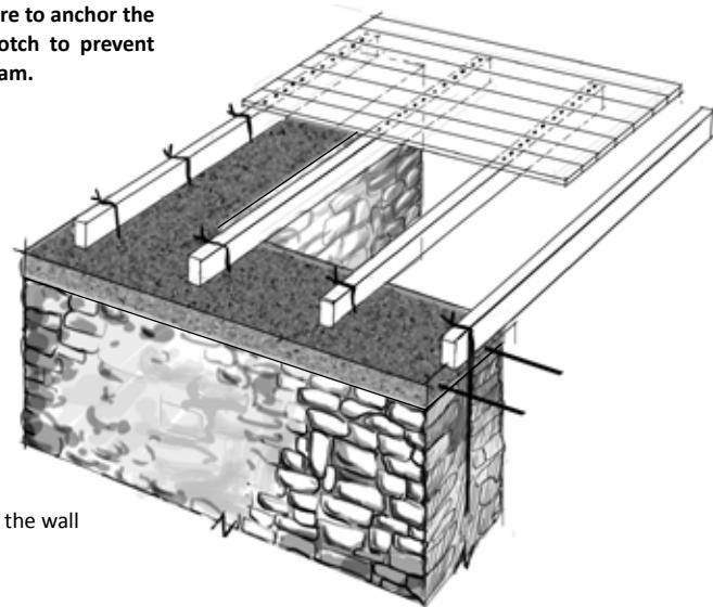
Figure 3.34 Tying floor joists to the wall
